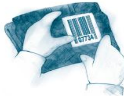
Bar codes are attached to the clothing to track it as it is assembled, washed, and prepared for shipment.
